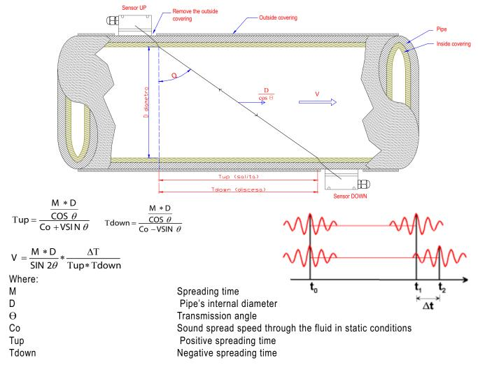
DT value is the difference of spreading time into a homogenous fluid without gas bubbles.
