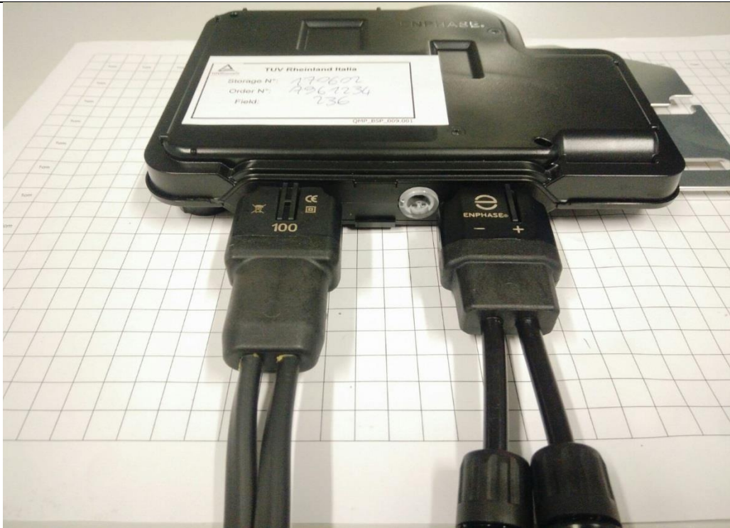
External View with cable AC and DC connected
