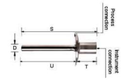
WELDED SANITARY CONNECT THERMOWELL
