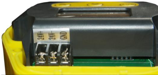
Wiring of electric (two-wire system)
