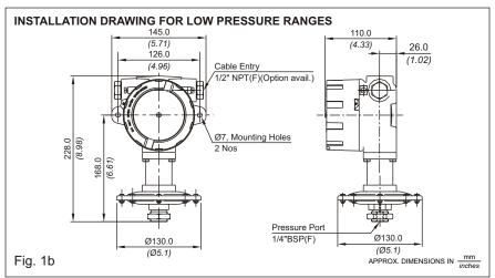
any direction . However , for low range pressure switches, it is advised to mount them in such a way that the diaphragm is vertical .
