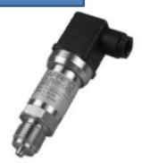
**Description:** Pressure transmitter convert physical pressure into an electrical signal proportional to the pressure. This Pressure Transmitter is equipped with a piezo – resistive silicon measuring cell.
