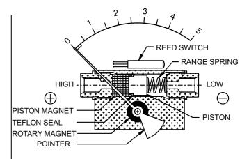
If pressure exceeds the rated maximum pressure, "O" rings used on male connectors, and the seal inside the pressure chamber, will be damaged. If maximum operating pressure is within the allowable limit, but the differentia I pressure exceeds instrument range, there will be no damage to the instrument. Pointer will only go to the extreme right end of the scale.
