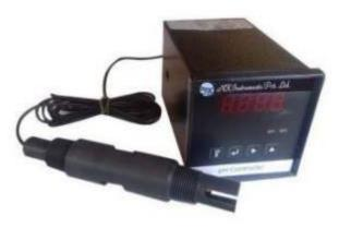
The Electrode being in glass material, is very delicate. We provide the Electrode Holder (guard) in PP as a standard. The same also can be provided in PTFE or, SS.
