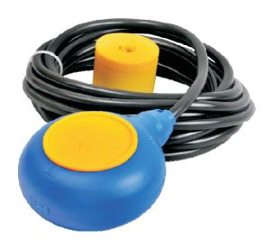
LSC is simple and reliable switch for level detection. It can be used for small or long range of storage tanks and reservoirs. Polypropylene rigid construction provides prevention from corrosion. Float tilt with liquid in rise & fall condition, accordingly micro switch operates from NO (Normally Open) to NC (Normally Close) position. It can be used as a multipoint switch also.
