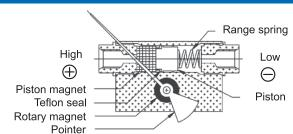
High and Low pressures are separated by **s**ensor assembly consisting of a magnet, piston, Teflon seal and a range spring. The difference in pressure causes the sensor assembly to move in proportion to the change against a range spring.
